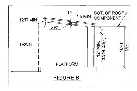
The bottom of roof components shall comply with the minimum height requirements of the International Building Code.
